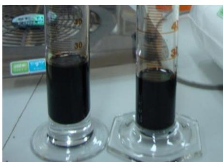
**Figure 2:** Photos of (left) CNSL extracted by using methanol and (right) *n*-hexane.
