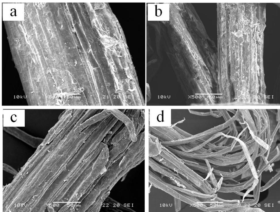
**Figure 2:** SEM pictures: (a) untreated SCB, (b) steam exploded SCB, (c) steam exploded SCB with xylanase treated and (d) bleached fibers
