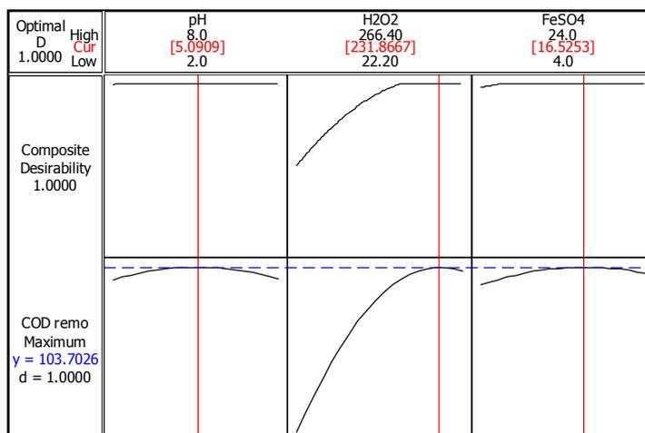
**Figure 2:** Response optimization of the COD removal efficiency (%)
