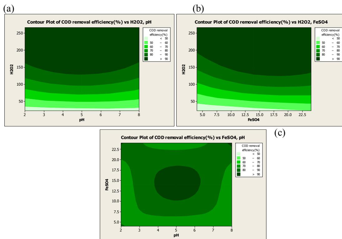
**Figure 1:** COD removal efficiency (%) correlating to (a) Interaction effect of H<sub>2</sub>O<sub>2</sub> and initial pH, (b) Interaction effect of H<sub>2</sub>O<sub>2</sub> concentration and FeSO<sub>4</sub> concentration and (c) Interaction effect of FeSO<sub>4</sub> concentration and initial pH
