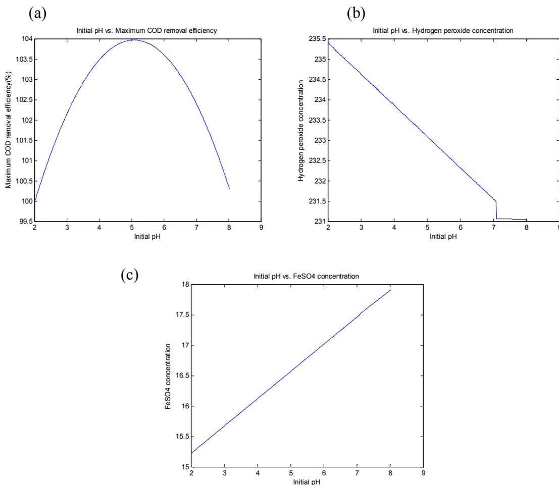
**Figure 3:** Interaction plotting of (a) initial pH versus maximum COD removal efficiency, (b) Initial pH versus  $\text{H}_2\text{O}_2$  concentration and (c) Initial pH versus  $\text{FeSO}_4$  concentration
